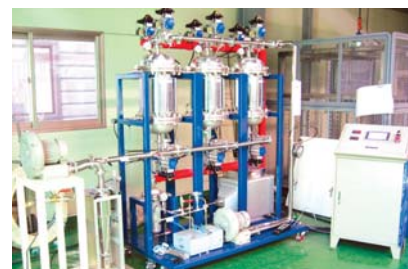
▲ VSA for recovering VOCs at Hyundai and Kia Motors' automobile painting shops (Pilot test facilities)
